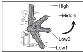
Use the head height adjustment lever (orange) to change the head height.
