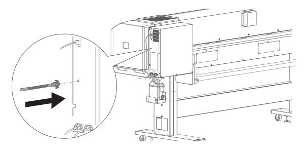
[3] Use the cable tie to secure the Ethernet cable to the printer.
