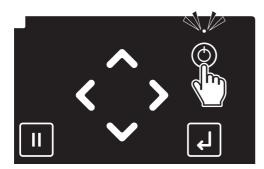
Press the power button on the control panel for more than two seconds.
