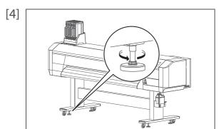
Loosen the four adjusters of Stand as shown in the left.
