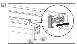
From the front side of the printer, pull the media feed lever towards you as much as possible to release the pressure rollers.
