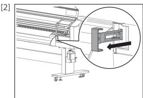
(To cancel the individual pressure rollers) From the front side of the printer, pull the media feed lever towards you as much as possible to release the pressure rollers.
