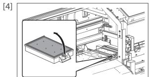
Pull the tab up of the absorption material for the flushing box, and release the hook.
